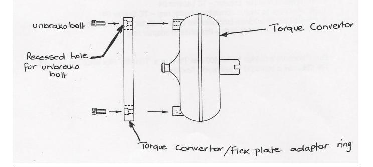
**Step 3:** Fit the torque convertor to the transmission. You will need to rotate the convertor and gently push it on until the measurement from them FACE OF THE TRANSMISSION to the FACE OF THE ADAPTOR RING that is bolted to the torque convertor measures 4mm behind the face of the transmission.
