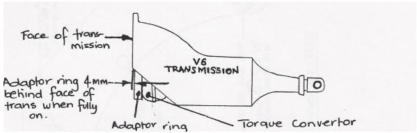
Step 6: The transmission fitted with the torque convertor can now be fitted to the motor using the bolts as shown on the main drawing. The torque convertor fitted with adaptor ring can now be bolted to the flex plate of the motor using the 3 off 3/8" UNC x 1" long bolts, rotate the torque convertor until all bolts fit. "Loctite type 242" would be of an advantage on these bolts as well.
